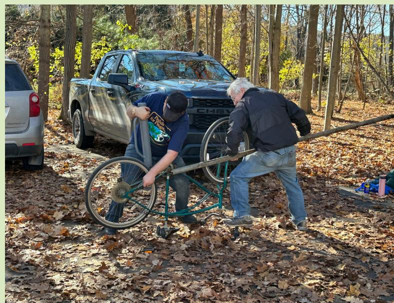
The three of them proceeded to slide the fence-post driver over the pedal wrench, then slide the pipe over the crank arm of the other pedal, then apply severe torque with the pipe. The creaking and aching noises of the pedal being released was the sweet sound of success.
